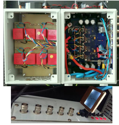
Fig. 3. DC-DC converter used for the PMSG connection to the DC Bus: inductors and capacitors box, PCB and connectors box, user interface
